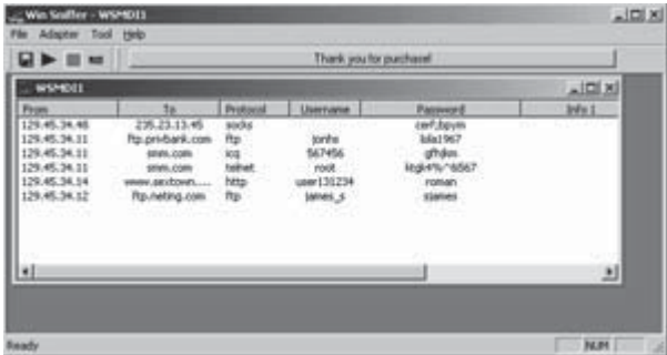
Figure 3-31 Win Sniffer pulls passwords from network traffic.
